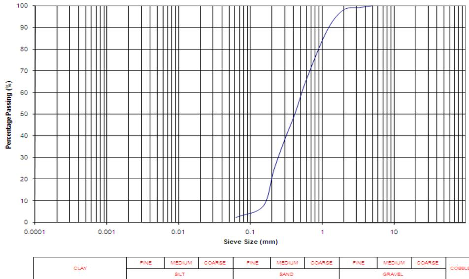
Fig.7: Particle Size Distribution Curve for BH-1
