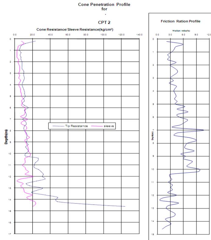
Fig. 3: Cone Penetration Profile (CPT of BH-2)
