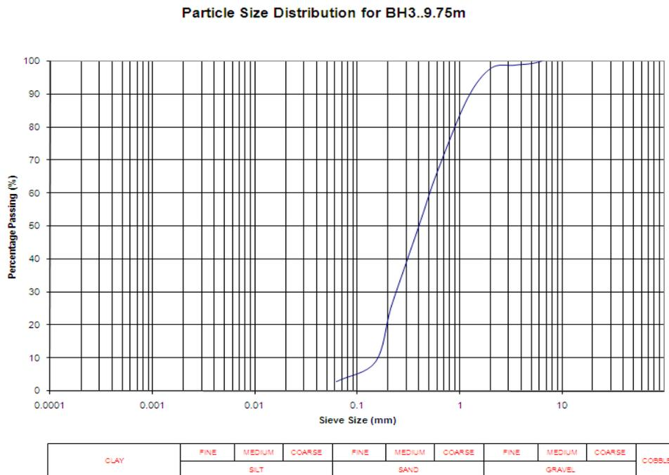
**Fig. 9: Particle Size Distribution Curve for BH-3**
