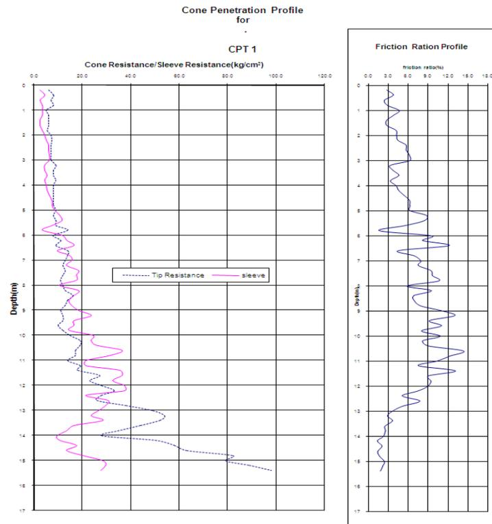
Fig. 2: Cone Penetration Profile (CPT of BH-1)
