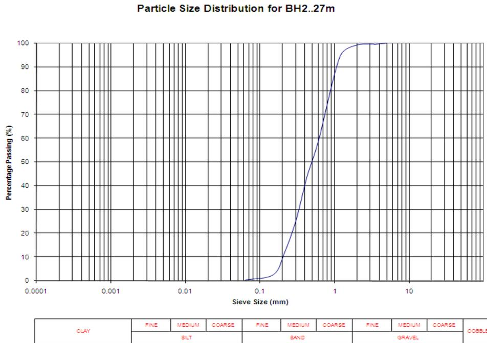
**Fig. 8: Particle Size Distribution Curve for BH-2**
