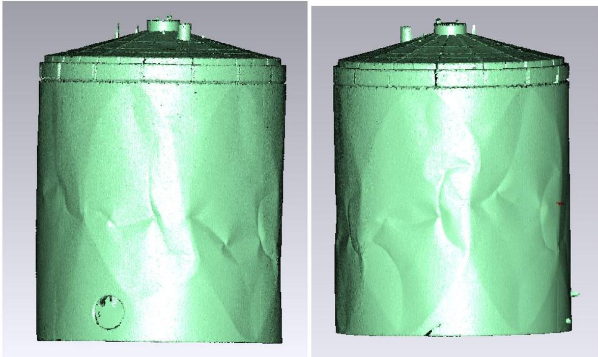
**Fig. 7: Point Cloud of the Surveyed Inner wall of the Damaged Tank**
