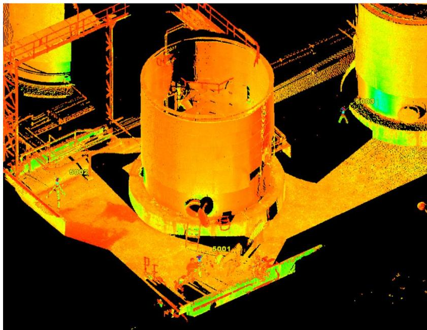
Fig. 5: Point Cloud of the Scanned Tank
