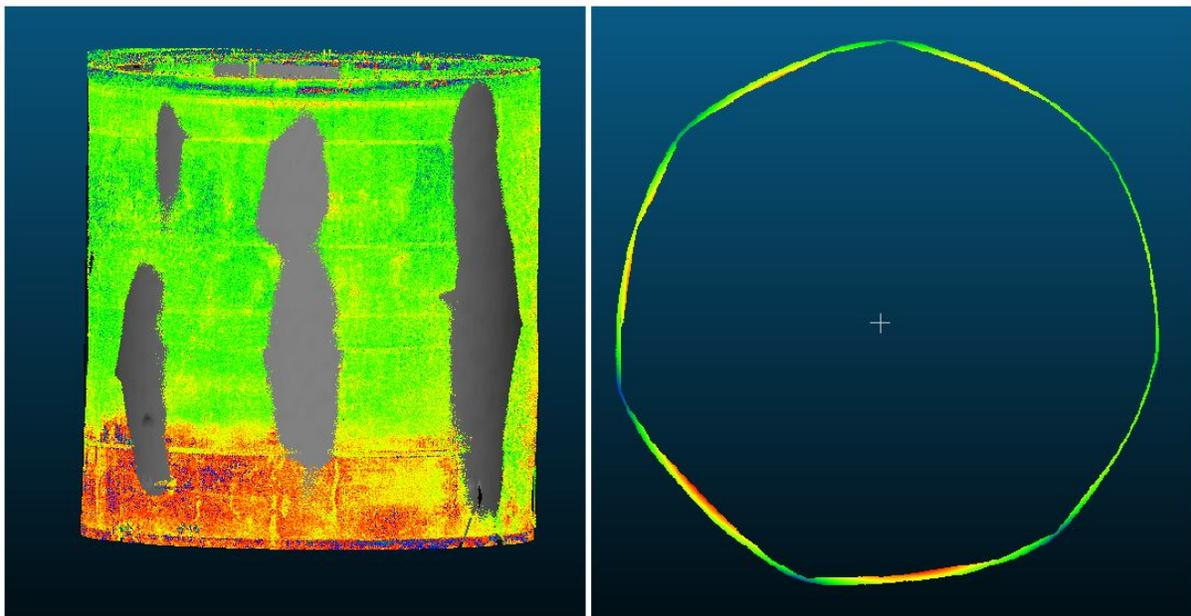
**Fig. 8: Identified Point Clouds of the deformed wall and the Reference Surface**
