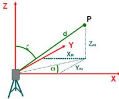
Fig. 4: The Principle of Spatial Polar Method [8,5]
