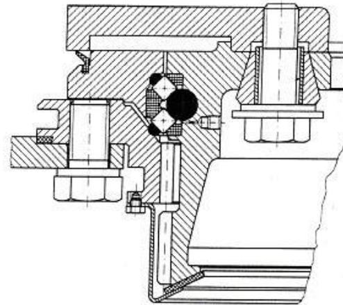
a) bearing attached to the contact surface with no prestress
