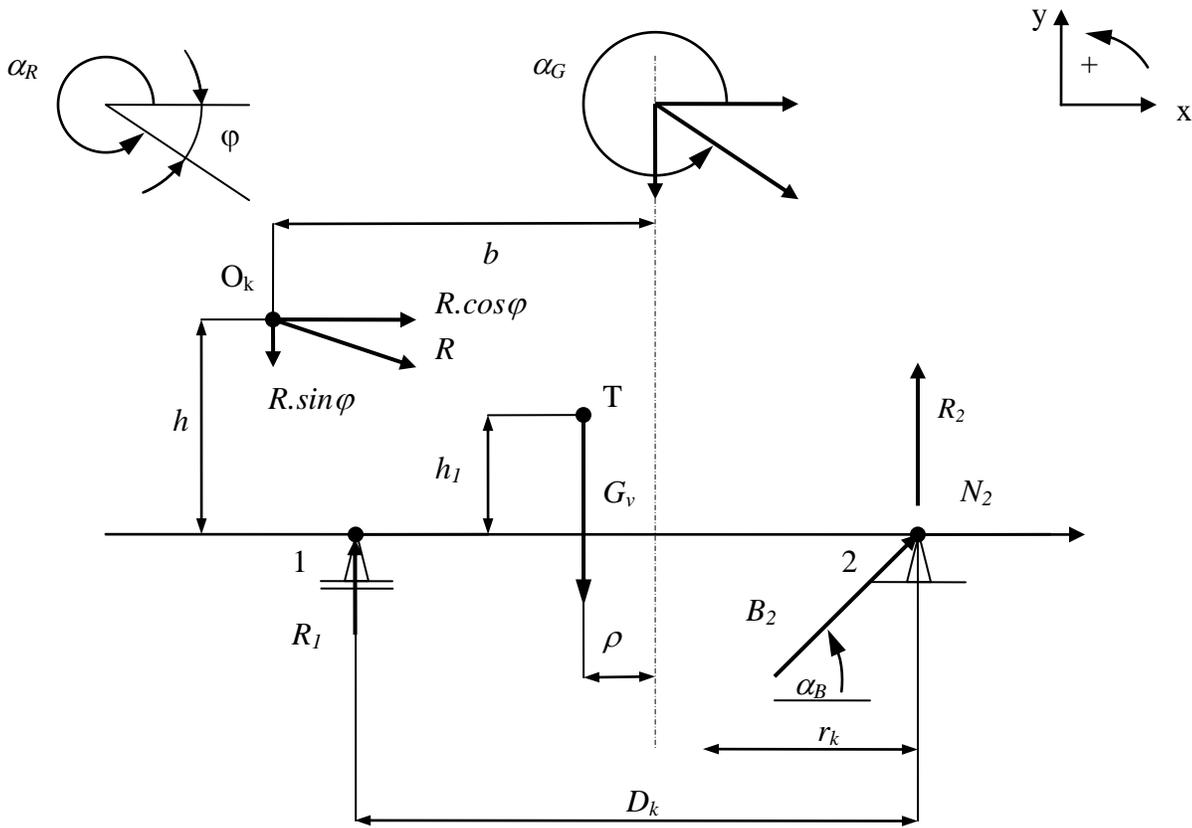
Fig. 3 Forces acting on the tank turret at the moment of firing from the tank cannon
