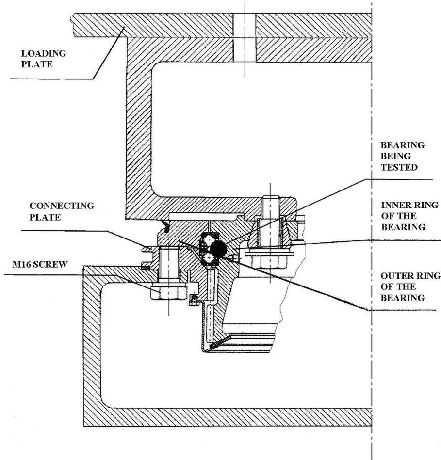
Fig. 5 Testing device for the T-72 M2 bearing
