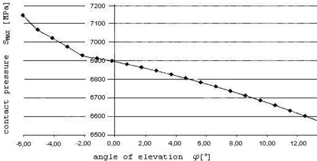
**Fig. 4 Dependence of the contact pressure on the angle of elevation of the cannon**
