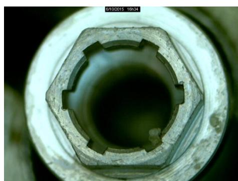
To extract the final measures of the deformations in the external hexagons (HE) of the dental implants in the study, individual photographs of the tested parts were analysed, and worksheets with the results were evaluated using Microsoft Excel.
