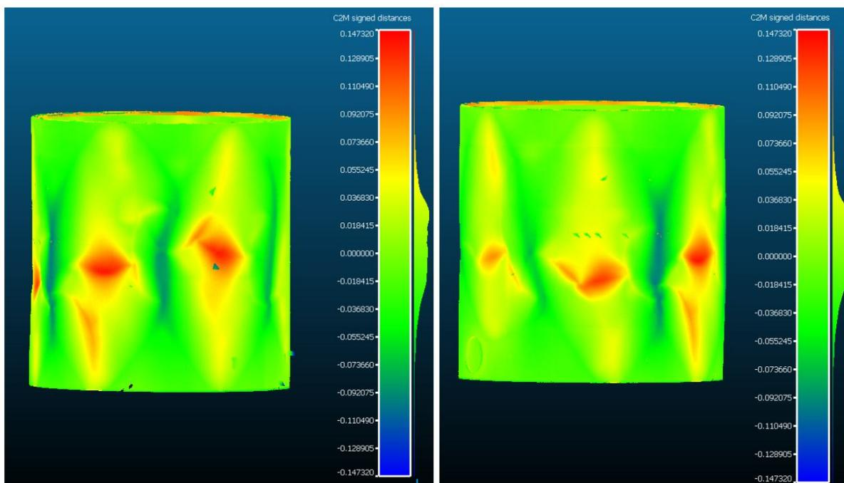
Fig. 9: Graphical Representation of Determined Deformations in the CloudCompare Software
