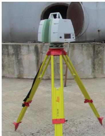
**Fig. 3: Terrestrial Laser Scanner Leica ScanStationC10**
