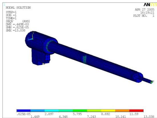
Fig. 4.11 Stresses inside the striker upon hitting the insert
