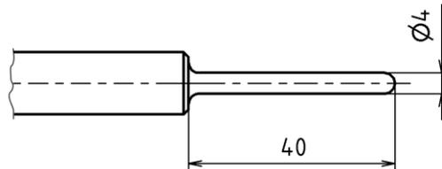
**Fig. 4.3 Firing pin****Calculation of the critical force**
