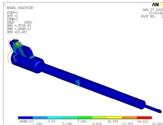
**Fig. 4.7 Hammer stresses in a stressed state of the rifle**
