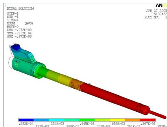
**Fig. 4.8 Hammer deformations in a stressed state of the rifle**
