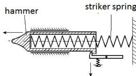
**Fig. 3.1 Striker mechanism with a hammer**
