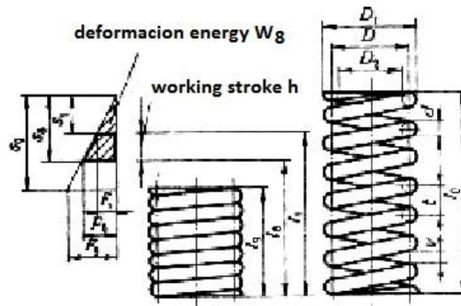
**Fig. 4.2 Characteristics of a compression cylindrical spring**
