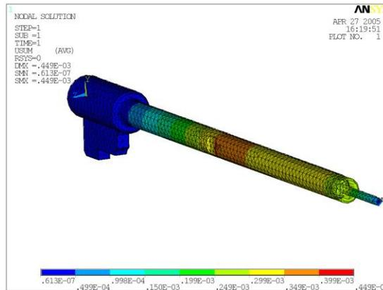
Fig. 4.12 Striker deformations upon hitting the insert
