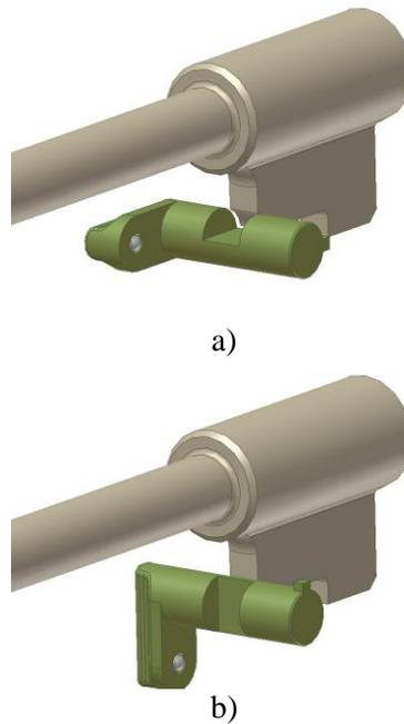
**Fig. 4.5 Hammer fuse and hammer**
