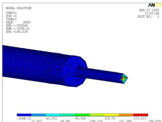
Fig. 4.9 Stresses inside the firing pin upon hitting the primer
