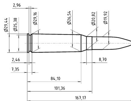
**Fig. 2.2** Fundamental dimensions of 20 x 102 mm cartridge
