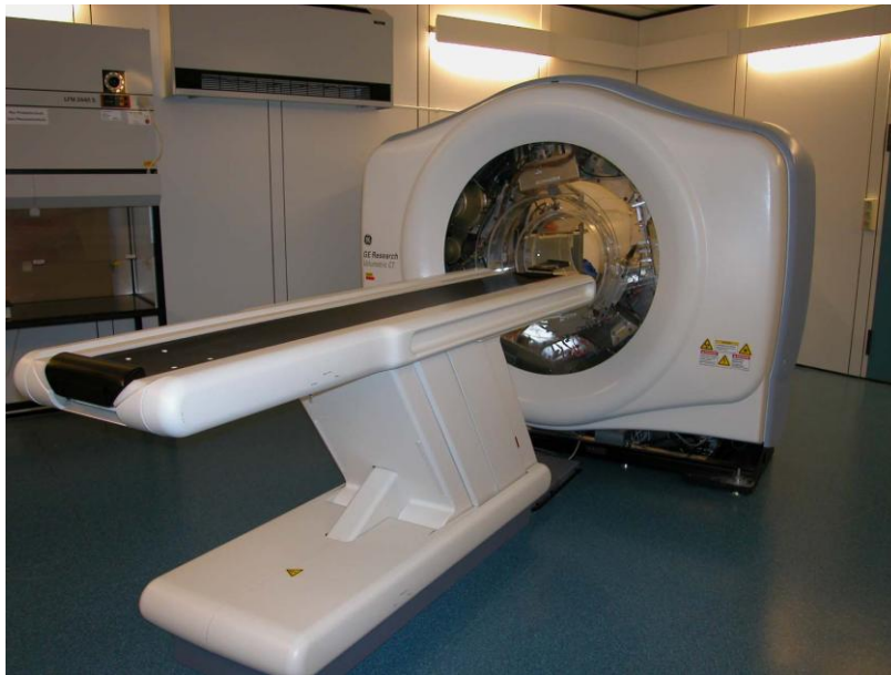
Fig. 3: Flat-panel detector-based volume computed tomograph (GE Global Research Center, Niskayuna, N.Y.)
